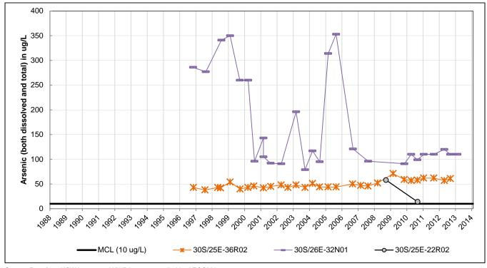
FIGURE 7.3-3B. Arsenic (50 - 400 μg/L) in Shallow Monitoring Wells - KWBA
