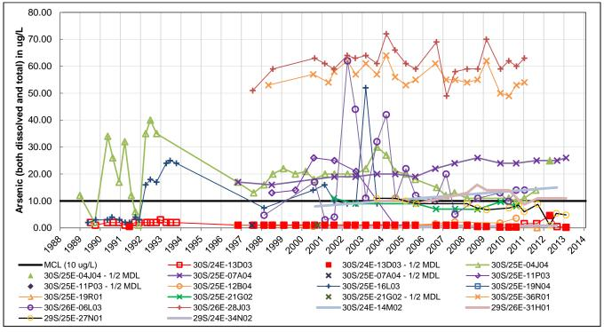
FIGURE 7.3-3C. Arsenic (from 0-80 μg/L) in Deep Monitoring Wells - KWBA
