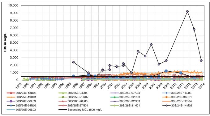
FIGURE 7.3-5C. Total Dissolved Solids in Deep Monitoring Wells with 30S/25E-12B04- KWBA
